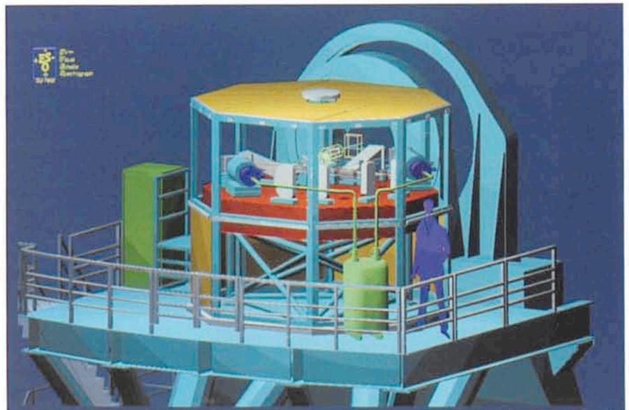
Figure 1: 3-D view of UVES with most of the enclosure panels removed for clarity.
