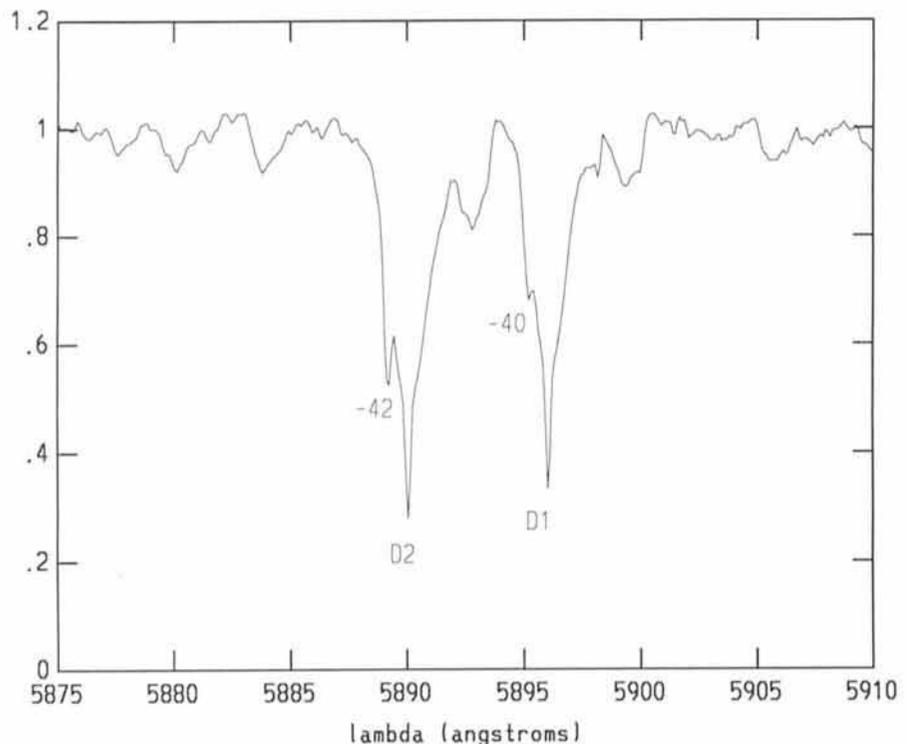
Figure 1: Normalized NaI D doublet of T Tauri star Sz 68. Radial velocities (in  $\text{km s}^{-1}$ ) of blue-shifted absorptions are relative to the interstellar component which is clearly recognizable in the stellar profiles.
