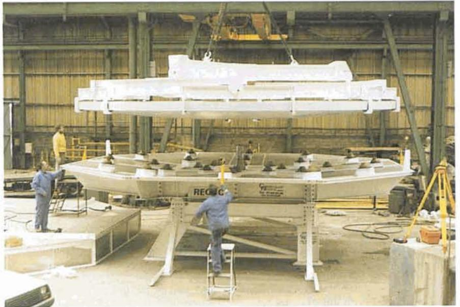
Figure 1: Dummy mirror being loaded onto the transport container.
