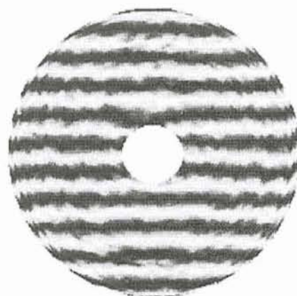
Figure 5: Synthetic interferogram calculated from the final phase map after stressed-lap polishing of the 3.5 m f/1.5 paraboloid. The measurement was made in December 1991 with a 633 nm phase-measuring interferometer through a refractive null corrector. The rms surface error is 21 nm (from Buddy Martin, Steward Observatory).
