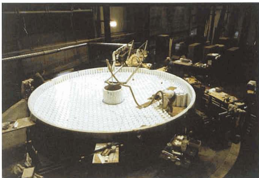
Figure 3: Preparation for fabricating the first 6.5-m borosilicate honeycomb mirror. The 6.5-m mould under construction. At the time of the Conference, the 6.5-m mirror had already been cast.
