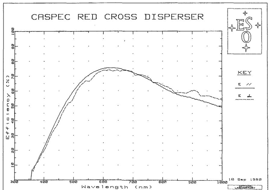
Figure 1: Efficiency curves for the RED cross disperser for polarization parallel and perpendicular to the grooves.
