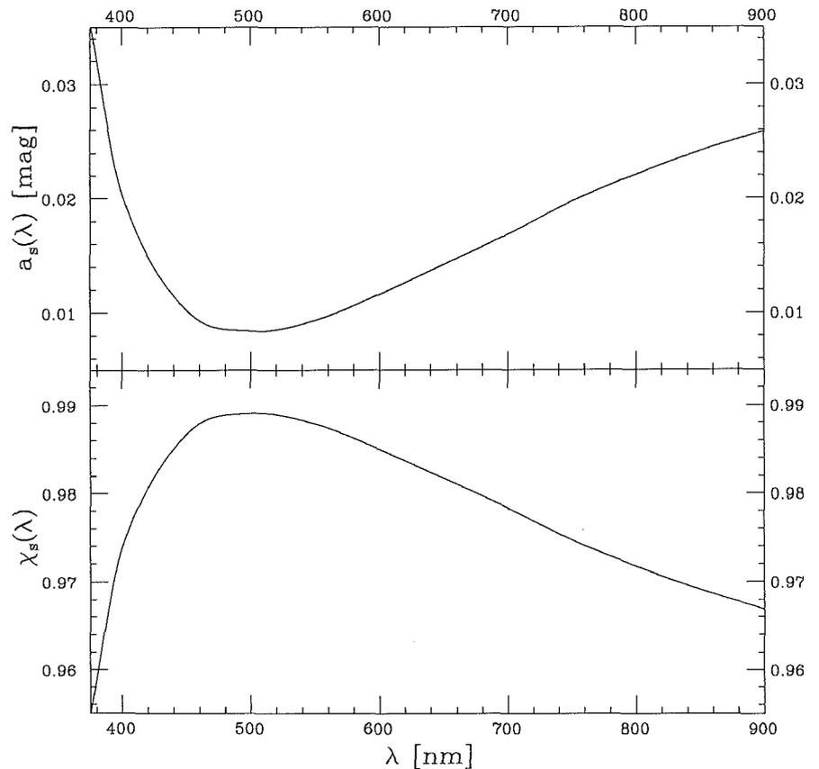
Figure 8: The total effects of differential atmospheric refraction, finite spectrograph-slit dimensions and slit orientation upon a stellar spectrum for a star  $z = A = 45^\circ$  with  $\sigma = 0'800$  and a horizontal mounted spectrograph-slit of sizes  $2a \times 2b = 5'' \times 240''$ . Top curve:  $a_s(\lambda)$ ; bottom curve:  $\chi_s(\lambda)$ .
