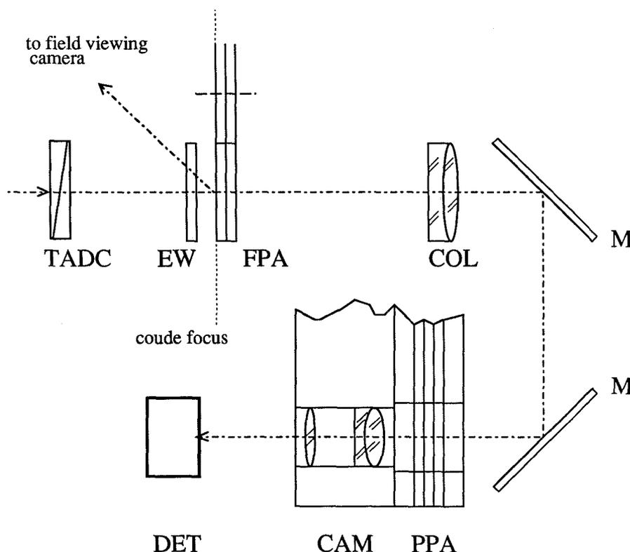
Figure 1: A schematic of the CONICA optical layout.
