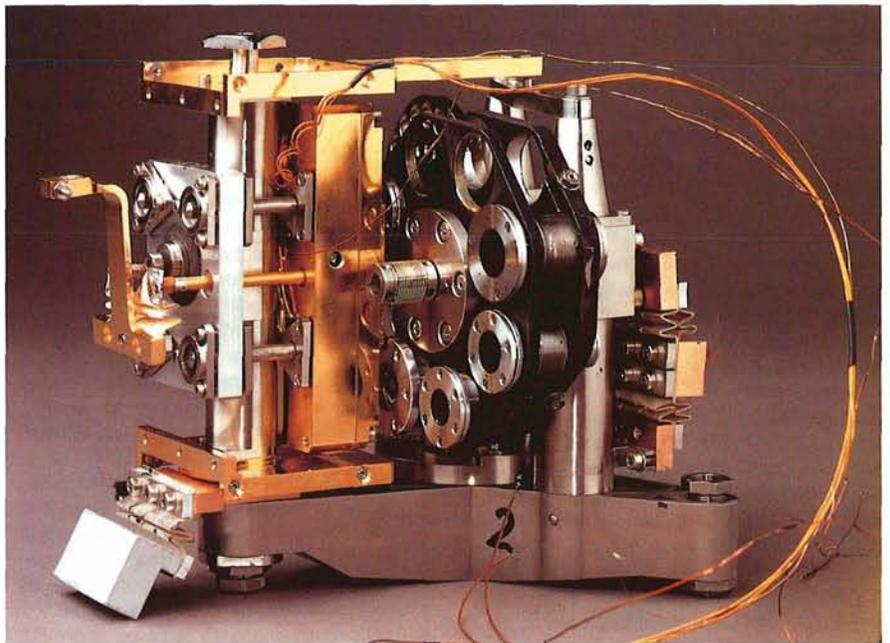
Figure 2: The cryogenically cooled optical assembly showing the array detector mount (gold), objective wheel and, just visible behind the latter, the 24-position filter wheel.
