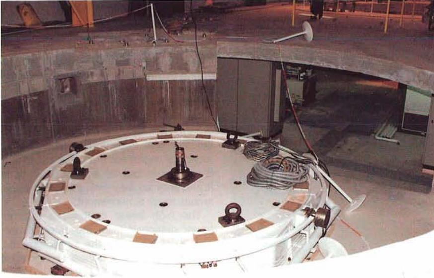
Figure 4: Base of the polishing rotating table installed in its pit. The oil pads at the periphery of the table base are protected by grey yellowish plastic. The track is attached to the table.
