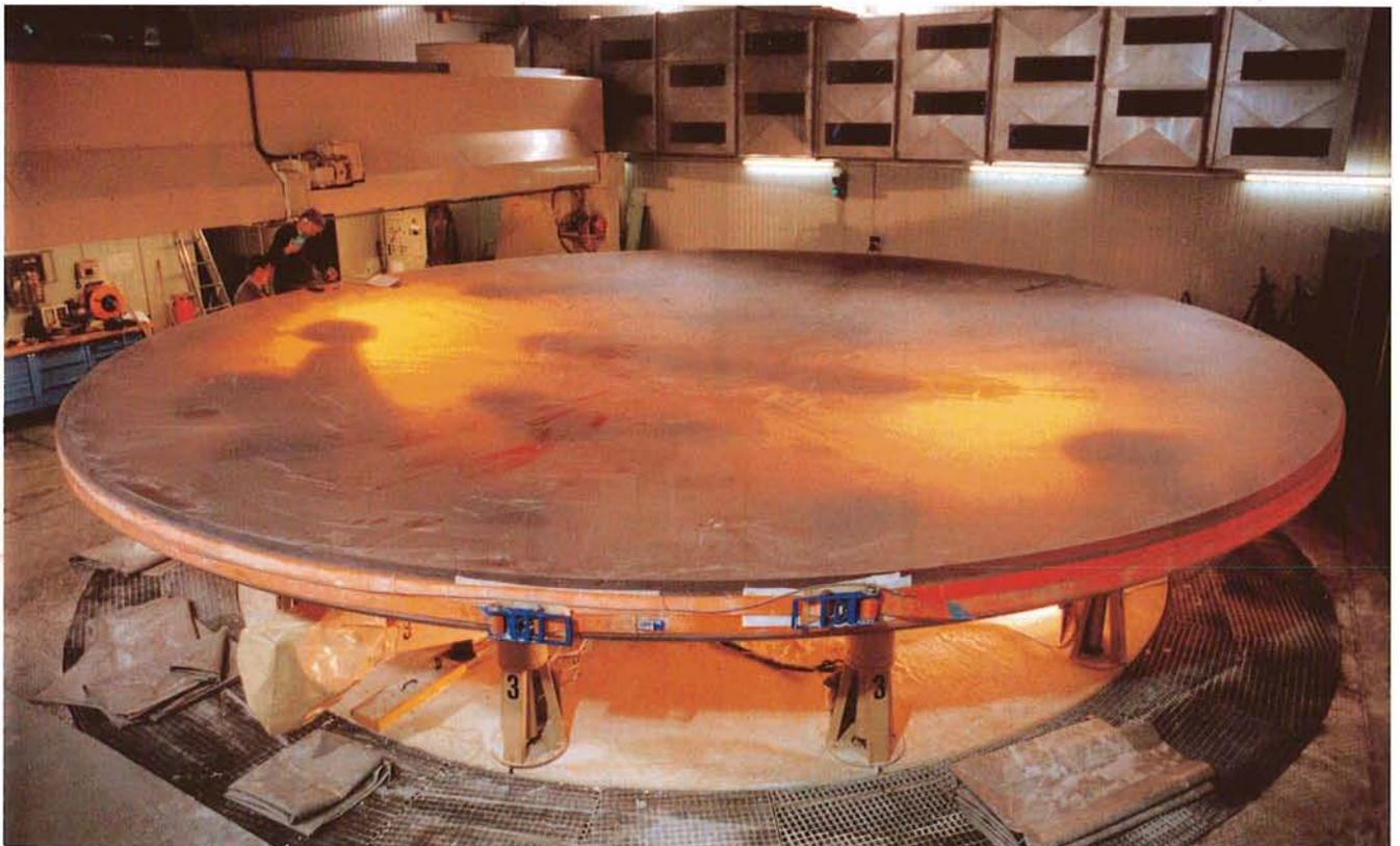
*This picture shows the first 8.6-m glassy ZERODUR-meniscus blank after machining at the SCHOTT factory in Mainz, Germany. This blank has been annealed, lifted from the mold, turned in a specially designed turning device and put on the 8-m CNC grinding machine. The blank is illuminated from below by two lamps; the yellowish colour is that of the glass. The yellow band around the blank is for protection during the machining.*
