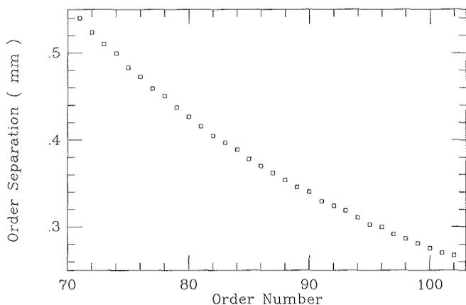
Figure 2: Interorder separation (in mm) vs. order number for CASPEC + short camera + 31.6 lines/mm echelle and RED cross disperser.
