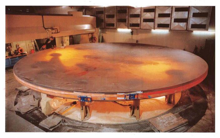
This picture shows the first 8.6-m glassy ZERODUR-meniscus blank after machining at the SCHOTT factory in Mainz, Germany. This blank has been annealed, lifted from the mold, turned in a specially designed turning device and put on the 8-m CNC grinding machine. The blank is illuminated from below by two lamps; the yellowish colour is that of the glass. The yellow band around the blank is for protection during the machining.
