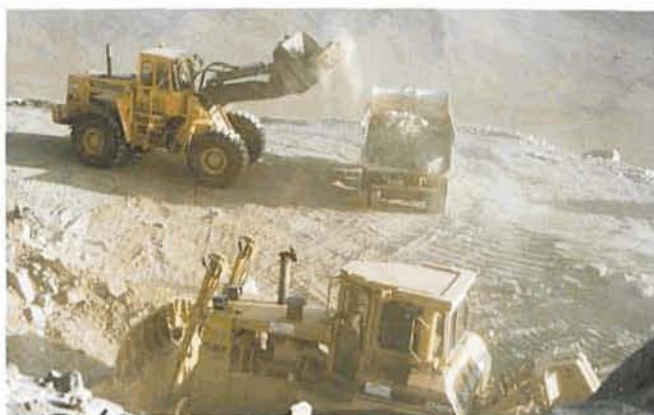
Figure 4: Excavation material loading.
