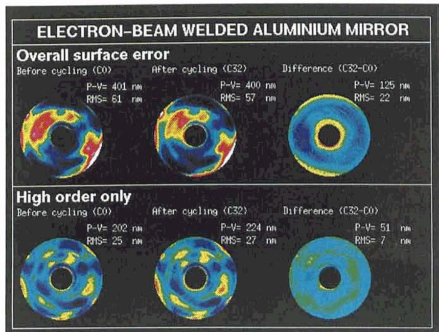
Figure 6: Surface maps of the EB welded mirror before and after thermal cycles.
