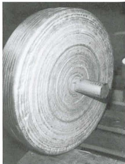
Figure 3: Build-up welded aluminium blank of 500 mm.
