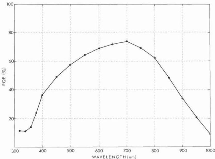
Figure 4: Quantum-Efficiency Curve of the thinned 1024<sup>2</sup> pixel TK CCD (ESO No. 23) now mounted on the SUSI direct-imaging camera.
