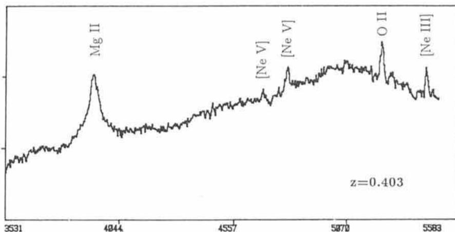
Figure 1: A blue spectrum of PKS0812+02 obtained with the NTT and EFOSC2 at a resolution of  $2\text{\AA}$  per pixel (Grism No. 3). The observation was done to check the feasibility of blue spectroscopy with a TH CCD (January 30, 1990; exp.:1800 s).
