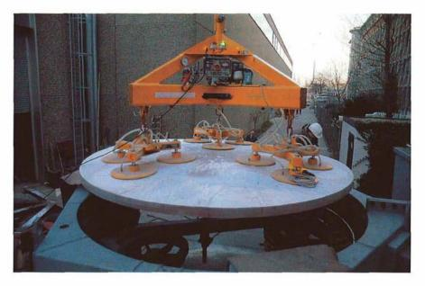
The picture shows the vacuum pumps located at the top and the large sucking cups arranged as a whiffle tree. The triangular structure is used as a vacuum buffer.
