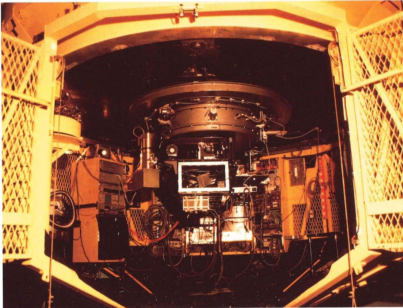
Figure 1: The adaptive optics prototype system installed at the f/8 focus of the 3.6-m telescope. The rectangular frame is part of the optical bench that supports the system. To the left of the bench is the IR array camera and on the right side is the wavefront sensor support. The electronics rack attached to the left side wall of the Cassegrain cage houses part of the front-end electronics of the system.
