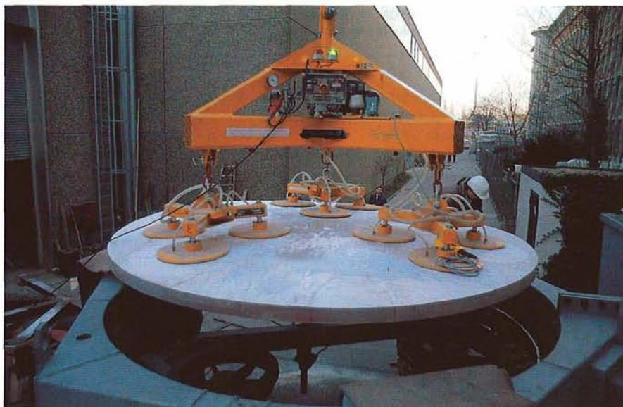
The picture shows the vacuum pumps located at the top and the large sucking cups arranged as a whiffle tree. The triangular structure is used as a vacuum buffer.
