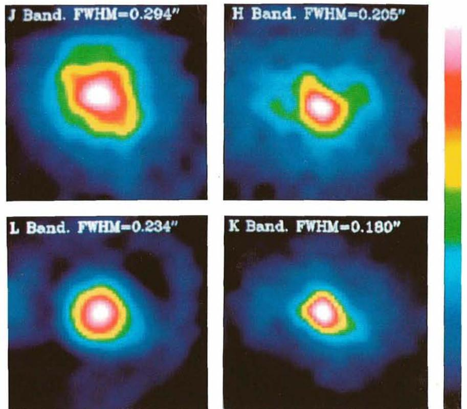
Figure 3: Imaging of the star  $\alpha$  Hydrae (HR 3748) in the J-, H-, K-, and L-Band with adaptive optics feedback. The dramatic image improvement is visible even in the J-Band where the system was undersampling at least by a factor of 2.5.
