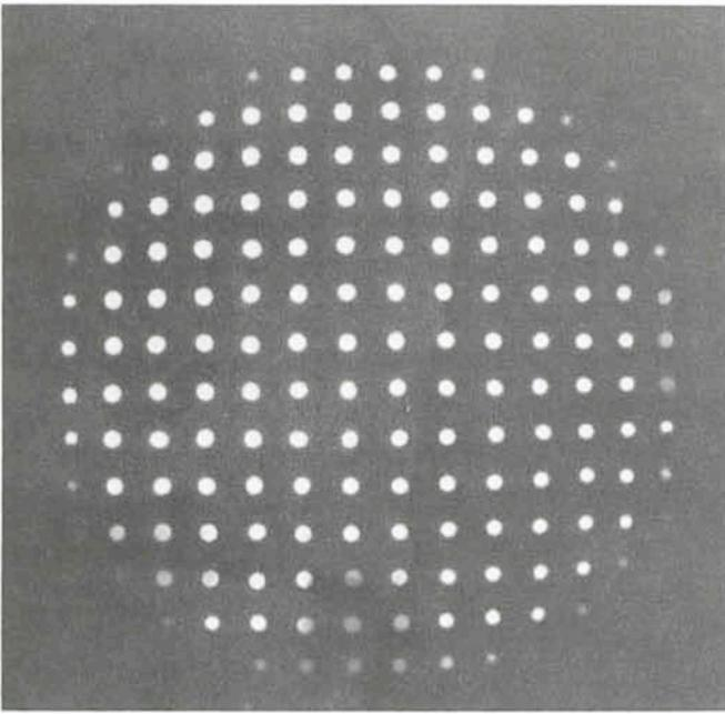
Fig. 1. Hartmann plate for  $f/5$  paraboloid of 600 mm diameter tested at centre of curvature.
