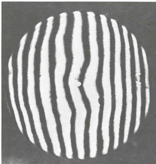
Fig. 2. Interferogram of same f/5 paraboloid tested at centre of curvature with compensating lens to remove spherical aberration.
