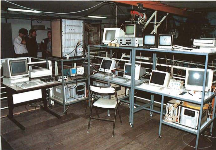
Figure 4: The control panel of the adaptive prototype system. The large rack in the upper left contains the wavefront computer. It is based on dedicated processors for a fast wavefront analysis.
