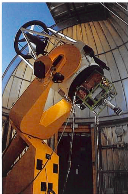
Figure 2: The Multichannel Photometer mounted at the 0.8-m DFM telescope.
