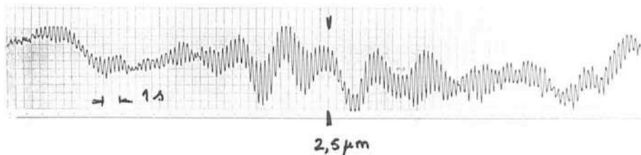
Figure 1: *Stability study at La Silla: The variation of the distance between the tops of the 3.6-m pier and the CAT pier at the base of each telescope, versus time, as measured with a laser interferometer, with a strong wind blowing outside. Horizontal axis: time; vertical axis: distance. A vibration appears at 5 Hz, but the stability of the distance is remarkable.*
