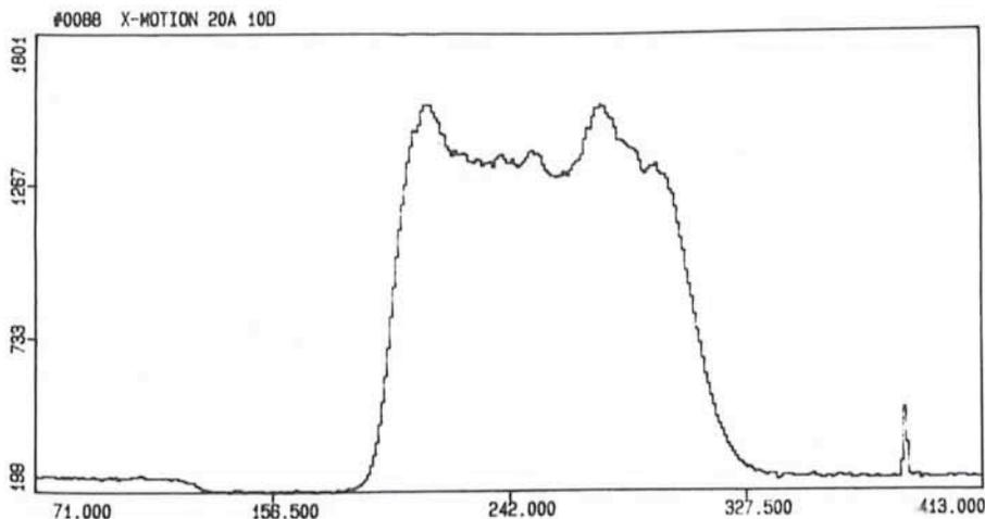
Figure 5: Calibration of the guiding motion of the telescope: A constant drift velocity  $d\alpha/dr = 20$  arcsec per hour and  $d\delta/dt = 10$  arcsec per hour is introduced and the signal from a star near Io is acquired during a 20-second exposure. The two-dimensional trail on the CCD detector provides the velocity scalings in  $\alpha$  and  $\delta$ . The intensity cut along the X-axis shows that the motion is not entirely uniform.
