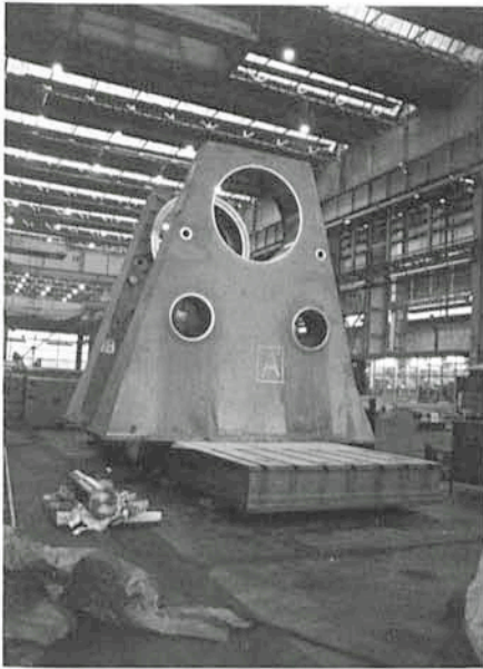
Figure 2: The fork arms on the reference plane. The seats (holes) for the drive units and for the big ball-bearing of the elevation axis are clearly visible.
