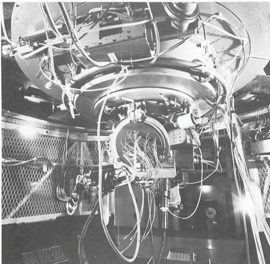
Figure 2: Wide angle view of OPTOPUS when installed in the Cassegrain cage of the 3.6-m telescope.
