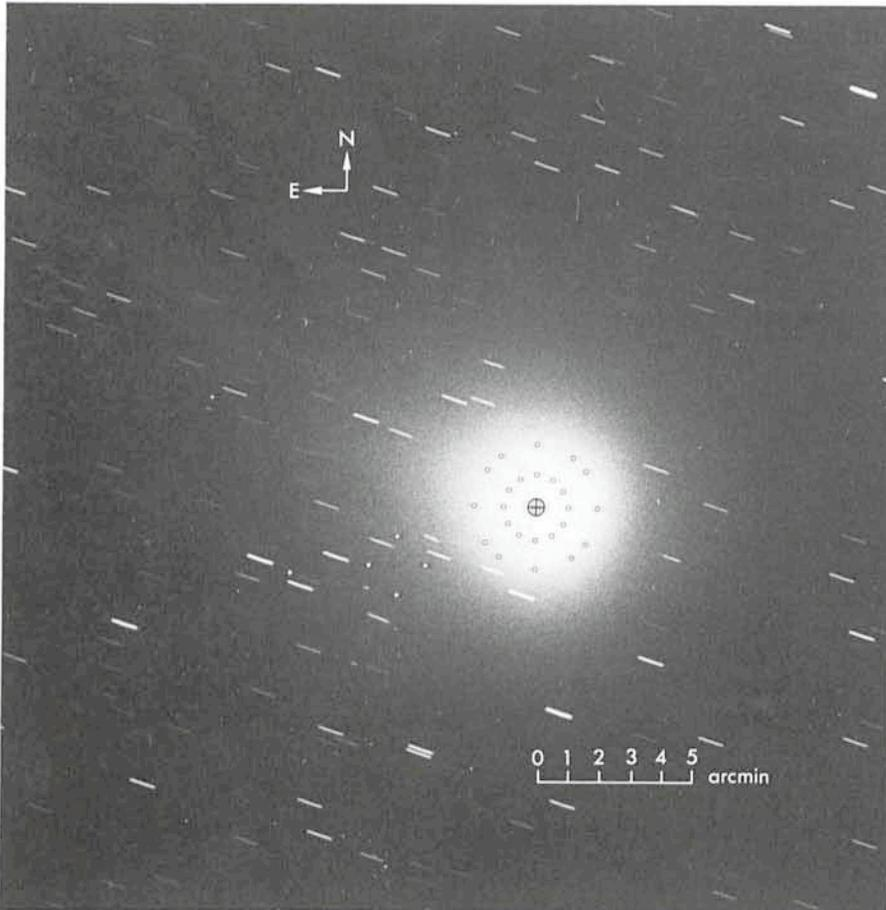
Figure 6: View of the central region of Halley's coma, with an overlay representing the locations in which the fibres were positioned. The outermost fibre positions are represented here with white spots, in order to distinguish them from the darker background. The central "crosshair" represents the coherent fibre bundle used for guiding. The detail visible in this print was made apparent by the use of a photographic masking technique described on page 12 in this issue of the *Messenger*.
