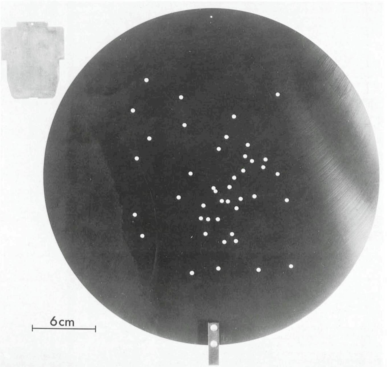
The giant and the midget: both attractive in their own way. In this picture, taken in the ESO Photolab, an OPTOPUS plate with holes to fit the optical fibers is shown close to a much smaller plate to be mounted on the EFOSC aperture wheel. Both combinations sample targets for multi-object spectroscopy at the Cassegrain focus of the 3.6 m telescope.
