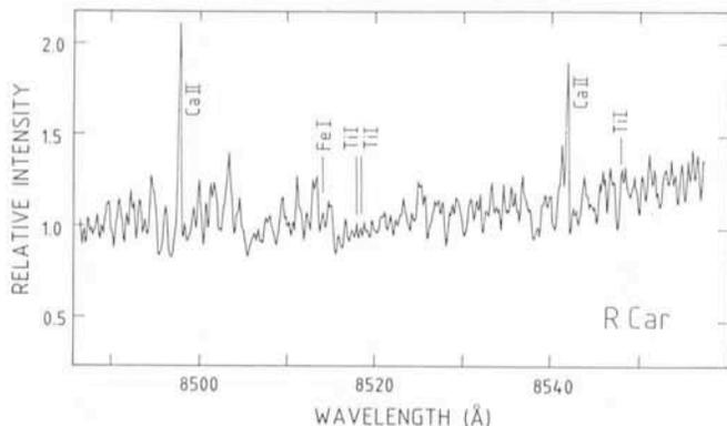
Fig. 3: Approximately the same wavelength range, resolution (85 mÅ) and signal-to-noise ratio (~200) as in Fig. 2 but for a typical Mira star (R Car) also near the luminosity maximum. Here, the molecular blends do not permit observation of the intrinsic line profiles.
