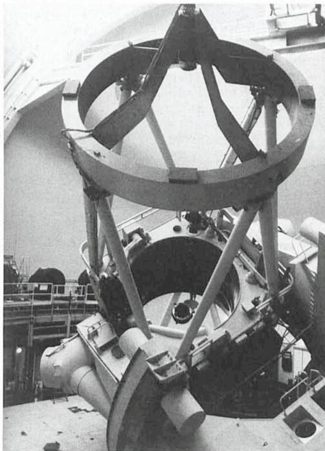
Fig. 1: F/35 top ring and chopping secondary mounted on the 3.6 m telescope.
