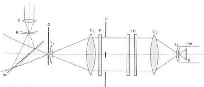
Fig. 1: Basic optical design of the spectrophotometer, showing principal components. E: eyepiece; R: reticle; M: mirror; D: diaphragm; L<sub>1</sub>: field lens; C<sub>1</sub>: collimating lens; F: filter; P: mask (image of telescope entrance pupil); FP: scanning Fabry-Perot; C<sub>2</sub>: imaging lens; L<sub>2</sub>: Fabry lens; PM: RCA C31034 photomultiplier; K: cathode.
