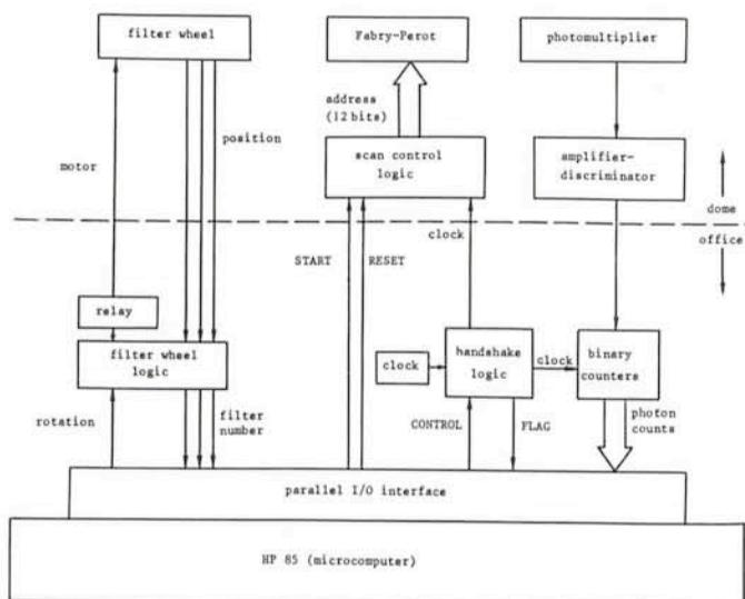
Fig. 4: Block diagram of the microcomputer control and acquisition system.
