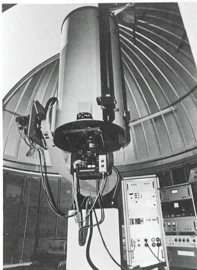
Fig. 1: The 70 cm telescope installed at La Silla in 1980. We notice on the optical axis the differential photometer which allows rapid sampling and on one of the Nasmyth focuses the photometer for occultations.
