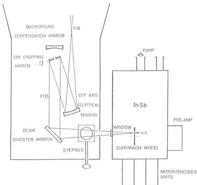
Fig. 2: Optical configuration of the IR photometer adaptor (see also 3.6 IR Photometer User's Manual).
