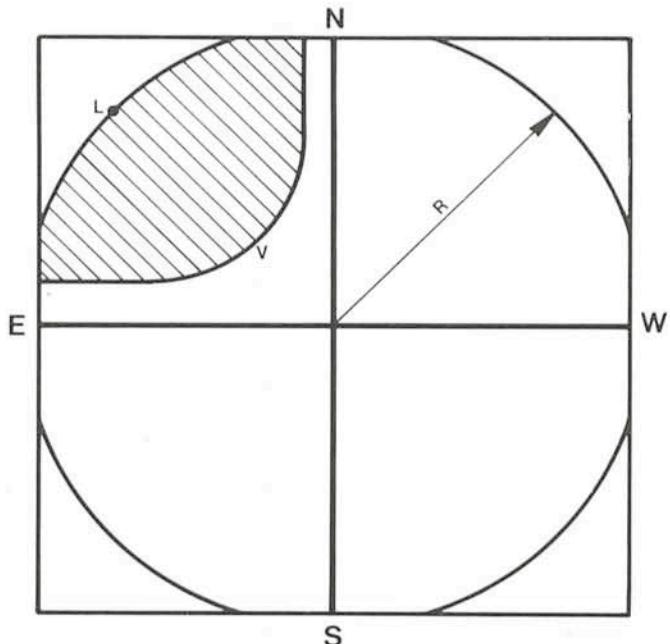
of the plate.  $R = 154.9$  mm. This means that for stars situated on the circle with this critical radius, the projection of the corrector plate on the mirror in the direction of the incident parallel beam is tangent to the circumference of the mirror. Stars outside this circle in the four plate corners are vignetted and cannot be used for photometry without special plate corrections.
