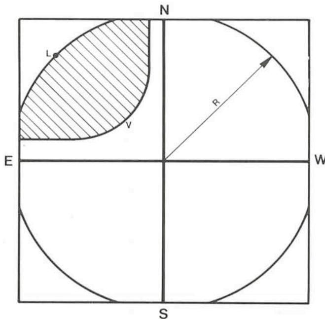
of the plate.  $R = 154.9$  mm. This means that for stars situated on the circle with this critical radius, the projection of the incident parallel beam is tangent to the circumference of the mirror. Stars outside this circle in the four plate corners are vignetted and cannot be used for photometry without special plate corrections.
