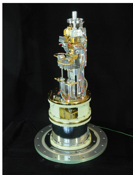
Figure 3. The ESO-led Band 2 receiver will be the first ALMA receiver compatible with the WSU requirements, covering an IF bandwidth from 2 to 18 GHz.
