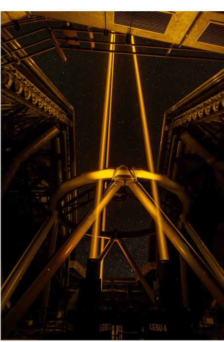
With advanced instruments designed to catch the light from extrasolar worlds and the Universe's most distant stars and galaxies, crystal clear images are a must. To achieve this, Unit Telescope 4 (Yepun) of ESO's Very Large Telescope (VLT) in Chile has an adaptive optics facility equipped with four sodium lasers, aimed towards the sky. When the laser beams reach about 90 kilometres into the atmosphere, they excite sodium atoms that start to glow, creating artificial stars in the sky.
