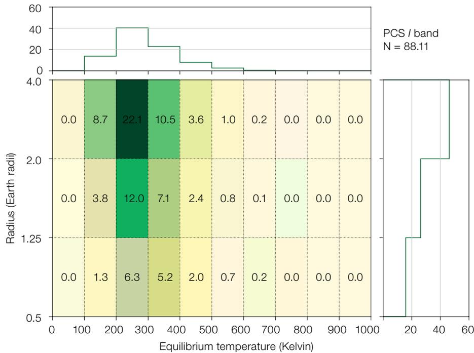
**Figure 5.** Number of small planet detections in the planet equilibrium temperature vs planet radius plane predicted for PCS observing in the  $I$  band at quadrature. The marginal histograms show the number of detectable planets as functions of temperature (top) and radius (right).
