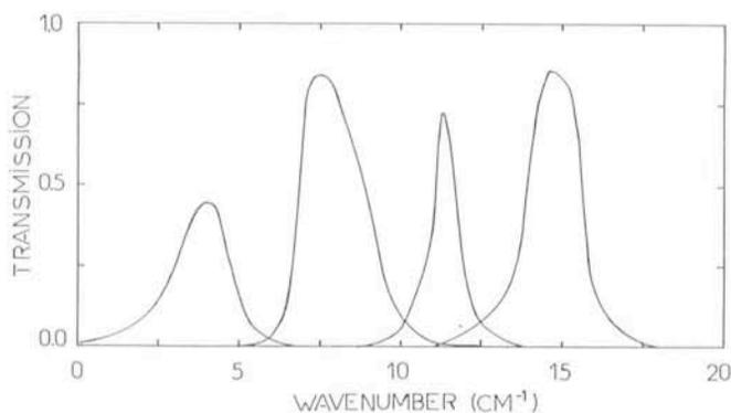
Fig. 2: Spectral shape of the band-pass filters used for astronomical sources.
