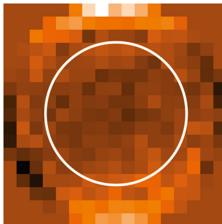
Figure 2. Real-time displays from the real-time computer. The left picture shows the Shack-Hartmann image. The four unused spots at the corners are vignettted at more than 50% by the pupil (represented by a white circle). The sub-apertures are represented in yellow. The picture on the right shows the voltage applied to the actuators of the deformable mirror, the white circle indicating the pupil footprint.
