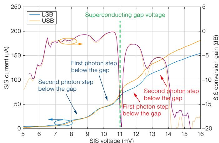
Figure 1. Plot of SIS current and conversion gain as a function of voltage bias for ALMA Band 3 at a local oscillator frequency of 100 GHz. The arrowed ellipses indicate the relevant ordinate: left for the SIS current and right for the conversion gain. See Shimojo et al. (2017a) for additional details.
