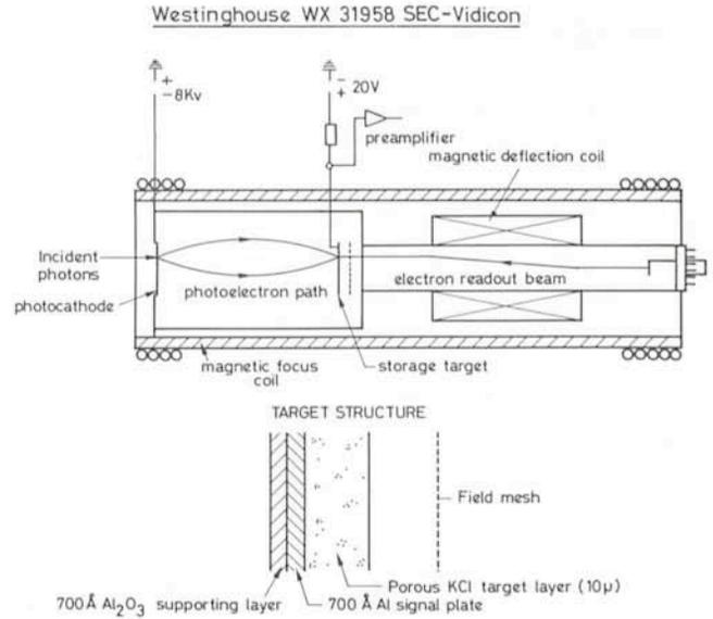
Fig. 2: Schematic drawing of the main parts of a SEC tube.
