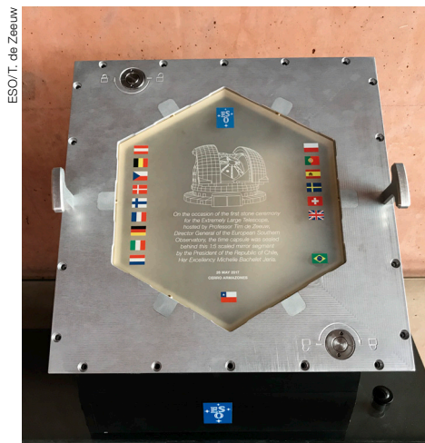
Figure 6. The time capsule that was filled during the ELT First Stone ceremony, manufactured at the Paranal mechanical workshop. The cover includes a 1:5 scale reproduction of a segment of the ELT primary mirror, made in Zerodur®.
