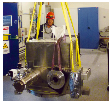
Figure 1. The MIDI cryostat is craned away from its base in the VLTI Laboratory after 12 years of productive work.
