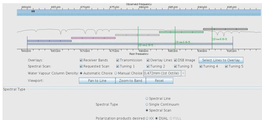
Figure 2. An example Observing Tool screen is shown for defining the spectral setup. In this example, a Band 9 spectral scan has been chosen, and the CO lines have been overlaid for visualisation.
