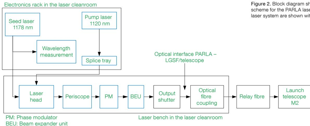
Figure 2. Block diagram showing the main optical scheme for the PARLA laser. The parts of the new laser system are shown with a blue outline.
