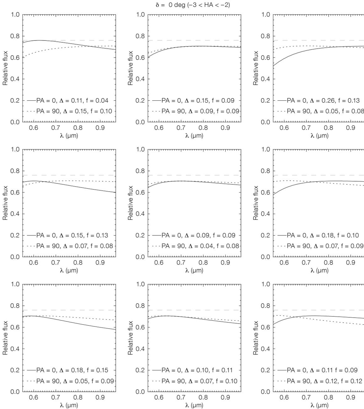
**Figure 2.** Output simulated spectra for nine different slit positions across the VIMOS FoV. These are the result of a one hour long integration ( $-3 < \text{HA} < -2$ ) on a  $\delta = 0$  degree field using the LR-red grism for an input flat spectrum. In each panel we show the spectra for two different slit orientations, as well as the corresponding relative flux loss ( $f$ ) and spectral distortion ( $\Delta$ ).
