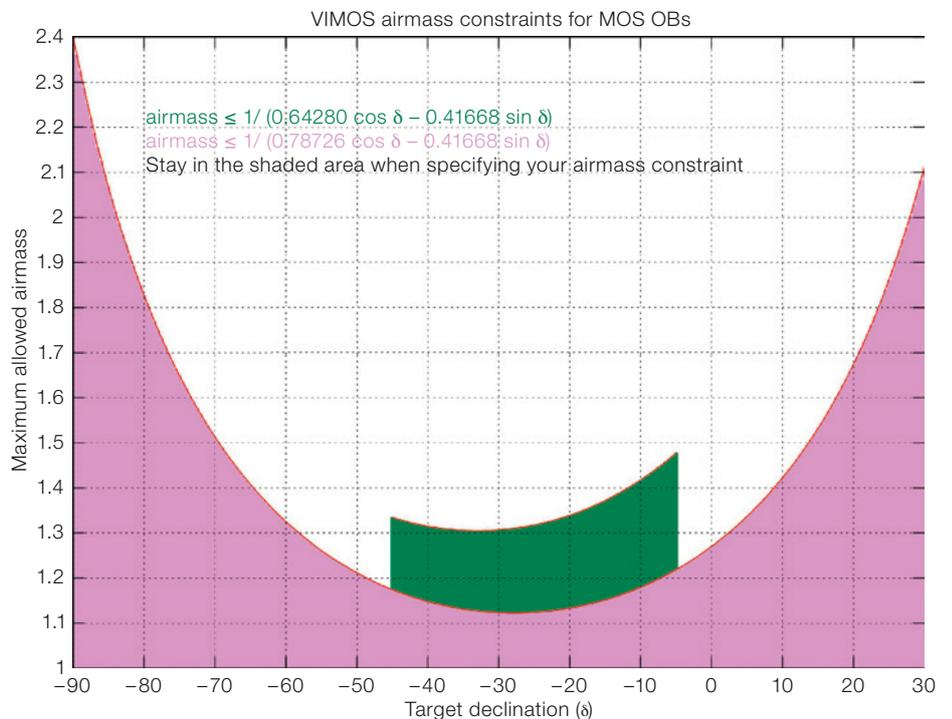
Figure 6. VIMOS airmass constraints for MOS observing blocks. The two different shaded areas correspond to the limits for fields that can be observed with slits having north–south orientations at meridian (purple), or east–west orientations (green). The generating formulae for these curves are shown with the same colour coding.
