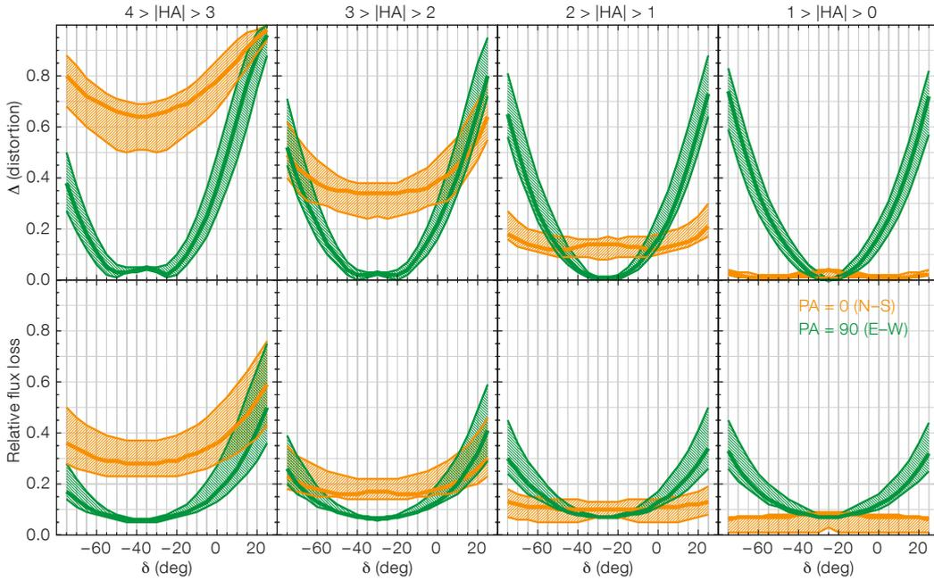
Figure 3. Curves show, for the LR-blue grism, the minimum, median and maximum flux losses (lower row) and spectral distortions (upper row) for the nine simulated slits as a function of target declination. The region between the minimum and maximum, about the median, is shaded. The plots show the effects for two different slit orientations at the meridian (north–south in orange and east–west in green).
