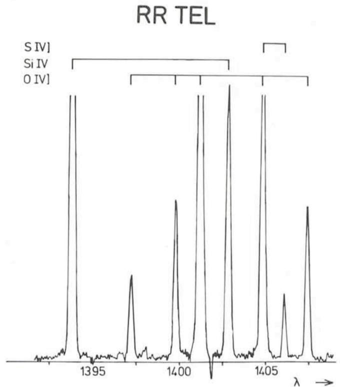
Fig. 4: A tracing of a portion of the "short-wavelength" UV spectrum of the slow nova RR Tel, showing the group of strong lines from O IV], Si IV] and S IV] near 1400 Å.
