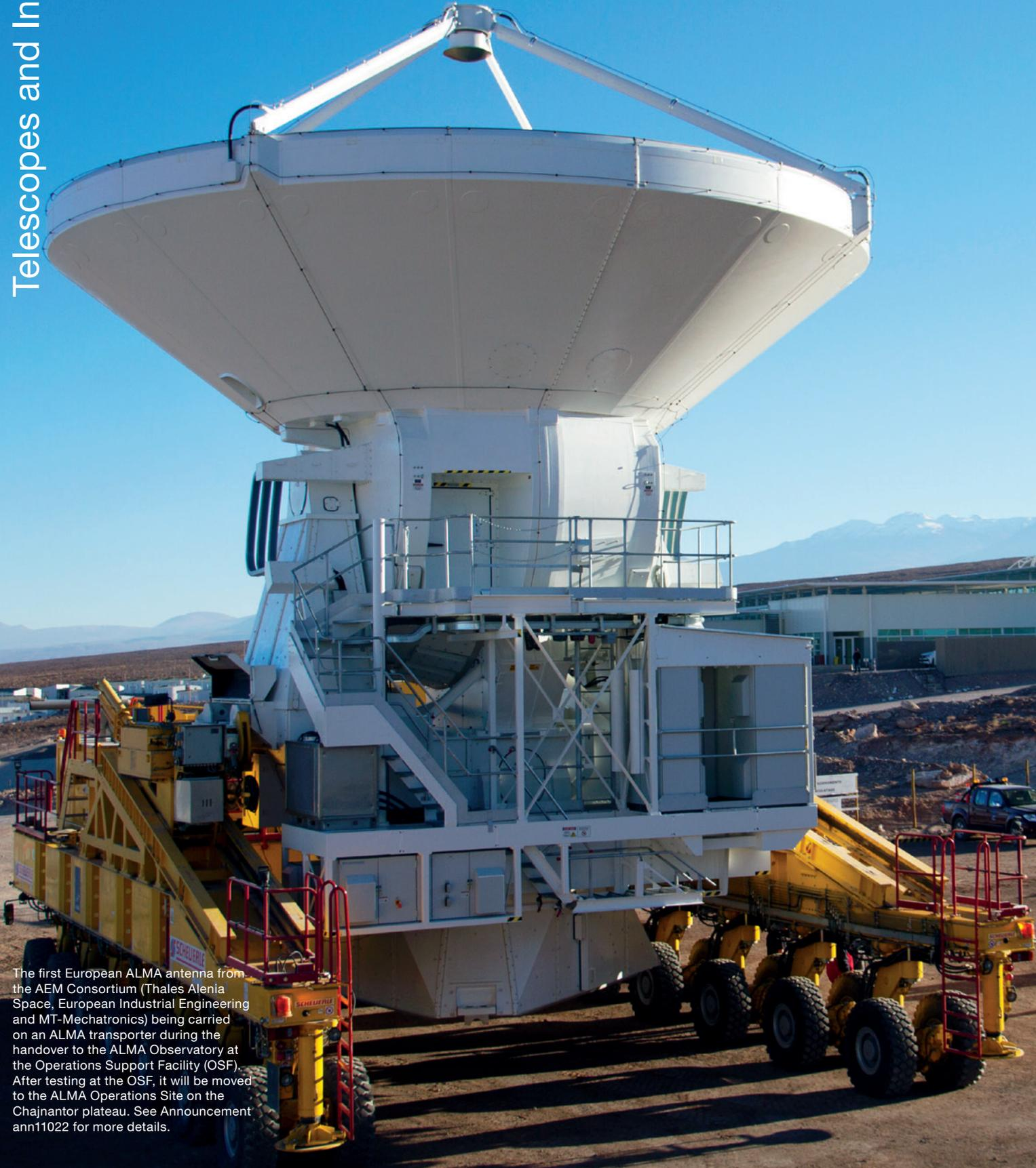
The first European ALMA antenna from the AEM Consortium (Thales Alenia Space, European Industrial Engineering and MT-Mechatronics) being carried on an ALMA transporter during the handover to the ALMA Observatory at the Operations Support Facility (OSF). After testing at the OSF, it will be moved to the ALMA Operations Site on the Chajnantor plateau. See Announcement ann11022 for more details.
