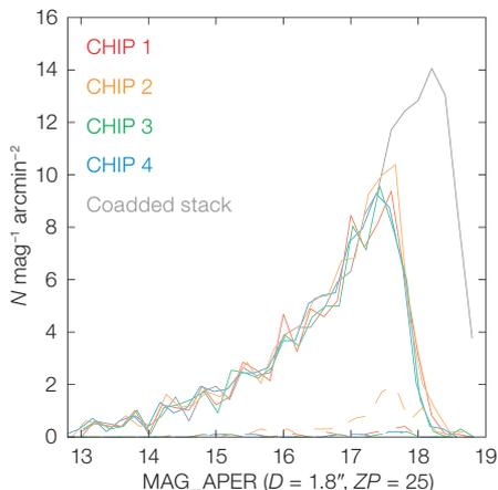
**Figure 2.** Number counts as a function of aperture magnitude of the four HAWK-I detectors: chip1 (red line), chip2 (orange), chip3 (green), chip4 (blue line) and the co-addition of all four chips (black line). Dashed lines give the number of spurious detections. Radioactive events are most common for chip 2, which nevertheless has a similar detection probability as the other chips, but an enhanced number of spurious detections at faint flux ( $> 17$  mag) levels (shown as dashed orange).
