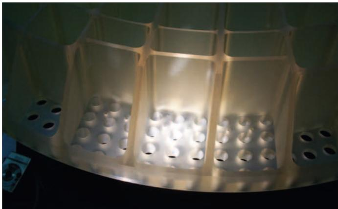
Figure 4. Part of the DSM reference body made by SESO in France (see the image on p. 4, upper, for the whole DSM). The intricate rib structure is literally sculpted from a monolithic block of Zerodur. The 1170 circular holes allow passage for the actuators. This process, known as lightweighting, reduces the mass by 80% to a mere 35 kg.
