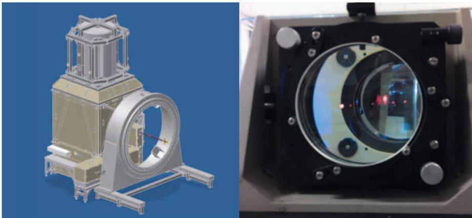
Figure 9. The ASSIST test bench (left) with the new generation M2 unit on top of the structure. The large 1.7-metre mirror is at the bottom (hidden by the light covers in this illustration) and the Nasmyth adaptor/rotator test bench can be seen on the right-hand side to allow the AO modules to be mounted. On the right is the secondary mirror (AM2), a 140 mm convex aspherical mirror manufactured by ASTRON, that completes the main tower optics of ASSIST.
