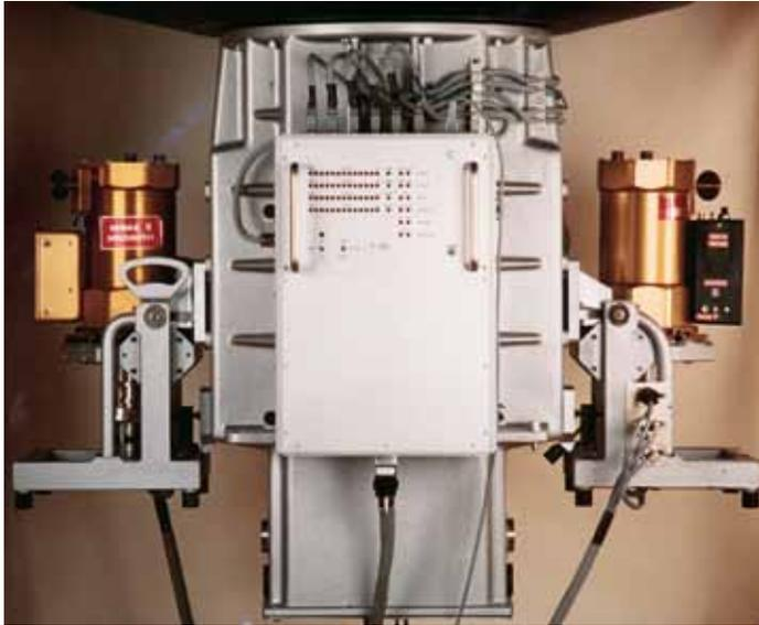
Figure 3. F/35 infrared spectrophotometers on the 3.6-metre telescope. The righthand dewar contains a liquid/solid nitrogen cooled InSb diode for 1–5  $\mu\text{m}$  photometry and the lefthand one a liquid helium cooled bolometer for 8–25  $\mu\text{m}$  photometry through broadband and narrowband circular variable filters. The support unit contains dichroic mirrors and a novel acquisition and guiding system using visible and IR TV cameras and a 2D tilting pupil mirror to explore the field.
