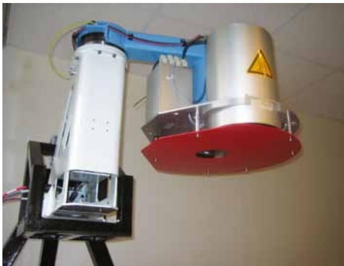
Figure 5. ACD#3 during PAI testing in the ESO ALMA laboratory.
