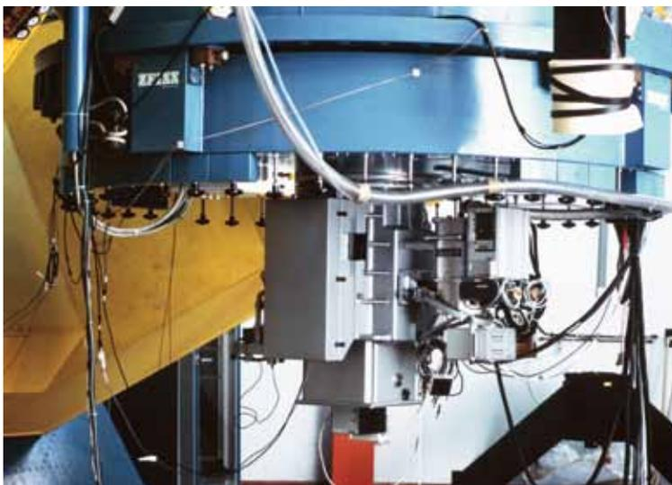
Figure 5. The F/35 IRAC1 camera mounted at the MPG/ESO 2.2-metre telescope.
