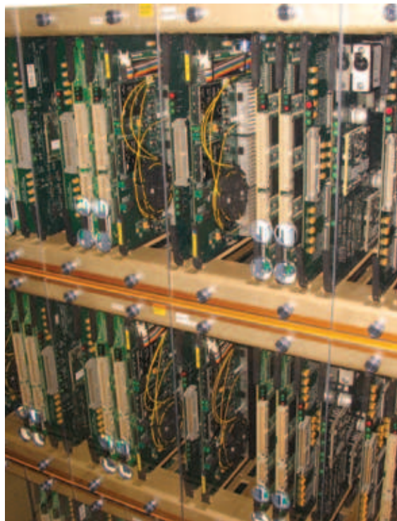
Figure 4. Front panel image of two bins in a Station Electronics rack showing TFB cards, station cards and other system cards (see Correlator Station Electronics in Figure 1). The pairs of holes seen in front of each TFB card allows cool air from the correlator room to be blown into the rack.
