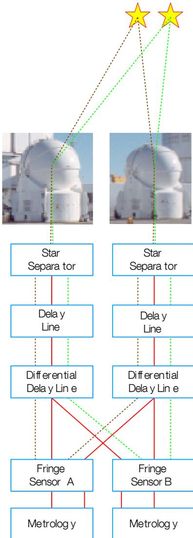
Figure 4. Schematic of the PRIMA system for the VLTI, highlighting the major subsystems along the optical paths of the facility.
