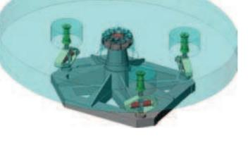
Figure 7 (below). CAD rendering of a Nasmyth platform populated with indicative instrument volumes and the prefocal unit.
