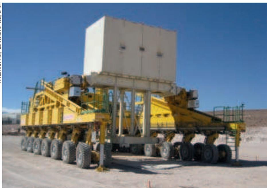
Figure 5. Transport with dummy load during loading sequence test.
