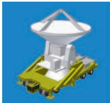
Figure 4. Transporter design with hydrostatically driven wheels.
