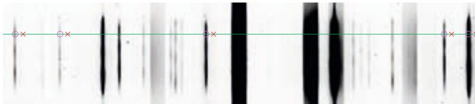
**Figure 2:** A CRRES full slit Th-Ar Hollow Cathode Lamp exposure used to discover the change in spectral format. The green line is the locus of a chosen entrance slit position on the detector array. Red crosses mark the predicted positions of isolated spectral features according to the baseline model parameter configuration. Purple circles mark the actual position of these features after a shift in spectral format.
