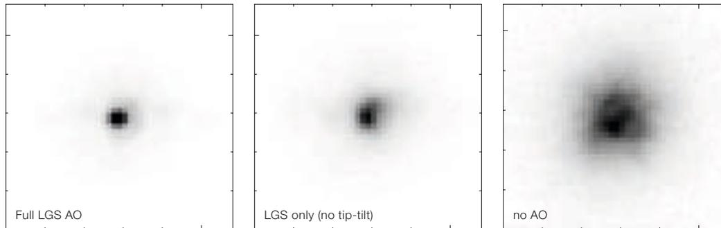
**Figure 1:** NAOS performance measured on CONICA in the *K*-band for full LGS-AO (left), and without tip-tilt (centre). The seeing limited PSF (right) is shown for reference. With full LGS-AO, the Strehl ratio was 22 % and the FWHM  $\sim 85$  mas. Without tip-tilt, the Strehl ratio was reduced to 10 % and the FWHM increased to 130 mas. For comparison, the *K*-band FWHM without AO is 300 mas.
