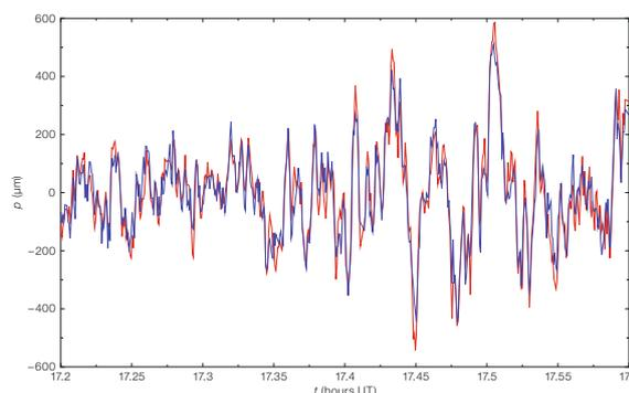
Figure 5: A sample of results from the Water Vapour Radiometer prototypes at the SMA. The red line is the fluctuating atmospheric path difference measured by the interferometer; the blue line is the best possible estimate from the radiometers.
