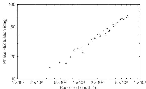
**Figure 2:** Measured phase fluctuations at the VLA at 22 GHz as a function of baseline length. The baselines shown in this plot are all between the antennas of one of the arms of the VLA and so are co-linear.
