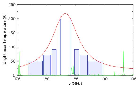
**Figure 3:** The brightness temperature of the 183 GHz water vapour line for a precipitable water vapour column density of 1 mm (red line) and the four double sideband channels of the prototype system (rectangles) with heights scaled in inverse proportion to bandwidth to illustrate their relative sensitivity. Also shown is exaggerated ozone emission (green lines).
