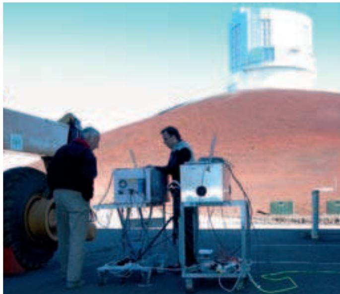
Figure 4: The two prototype water vapour radiometers on Mauna Kea, in initial tests before installation on the SMA.
