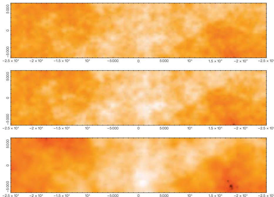
Figure 1: Maps of vertically integrated models of water vapour content generated assuming three-dimensional Kolmogorov statistics. The three maps (top to bottom) correspond to increasing vertical thicknesses of the turbulent volume showing the expected steepening (i.e., increasingly more power on the larger scales) of the fluctuation structure function. The horizontal dimensions of the maps are 50 km  $\times$  14 km and the resolution is 24 m.
