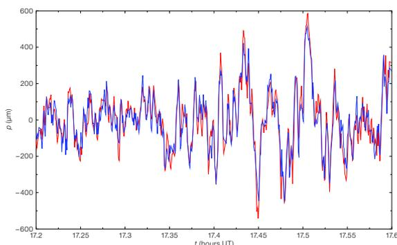
Figure 5: A sample of results from the Water Vapour Radiometer prototypes at the SMA. The red line is the fluctuating atmospheric path difference measured by the interferometer; the blue line is the best possible estimate from the radiometers.
