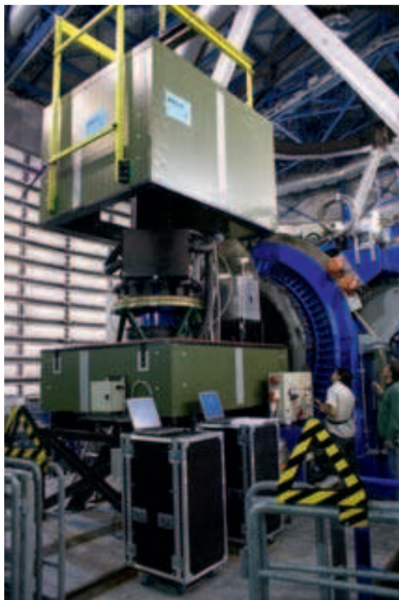
Figure 1: DAZLE being mounted on the VLT UT3 (Melipal) visitor focus.
